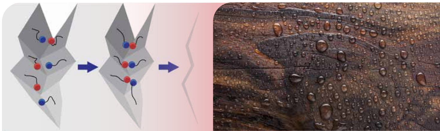
Figure 1.0 Self-healing process induced by reversible interactions
